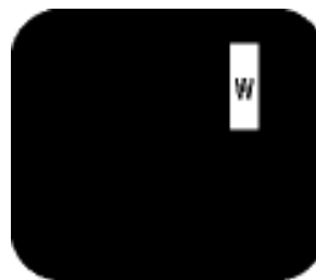
Three adjacent lit subpixels (one white pixel)
