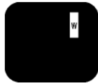
Three adjacent lit subpixels (one white pixel)
