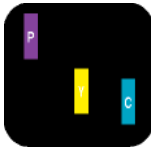
Two adjacent lit subpixels: - Red + Blue = Purple - Red + Green = Yellow - Green + Blue = Cyan (Light Blue)
