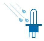
Only a burning bulb made of quartz glass (filament 2650°c, glass 800°c) can resist thermal shocks: such as, if a drop of cold water touches the hot bulb, which can happen when you drive through water with a broken headlight unit. ^Application varies per bulb type
