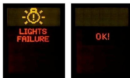
LED bulb Canbus NOT compliant LED bulb + CEA5W Canbus compliant
