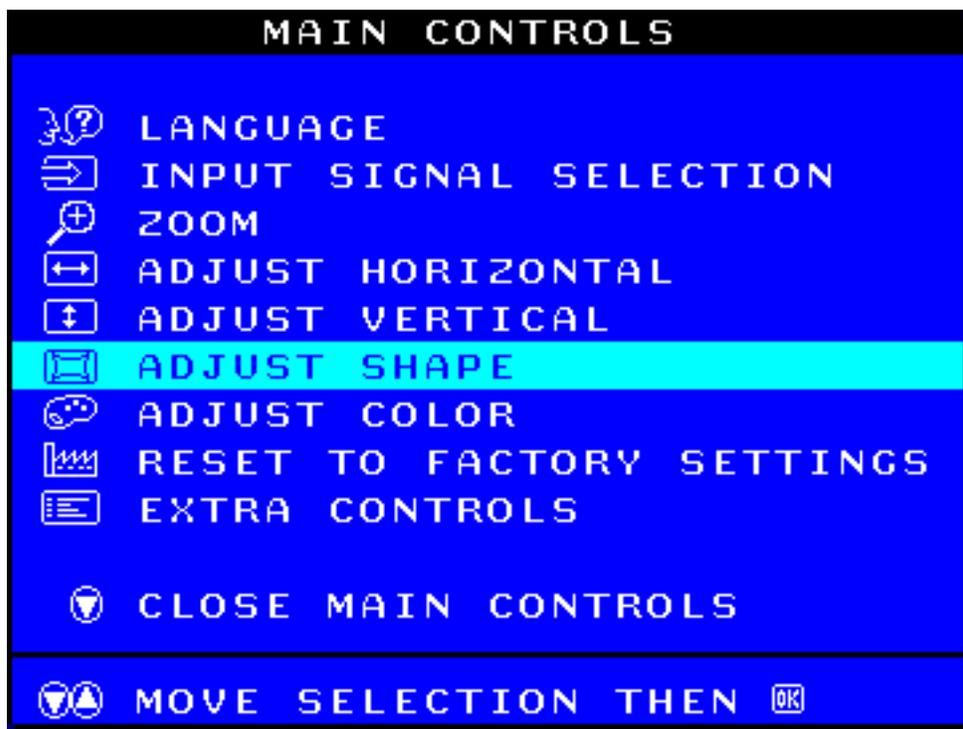
3) Press the
