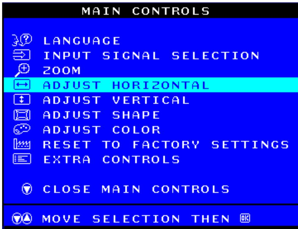
3) Press the
