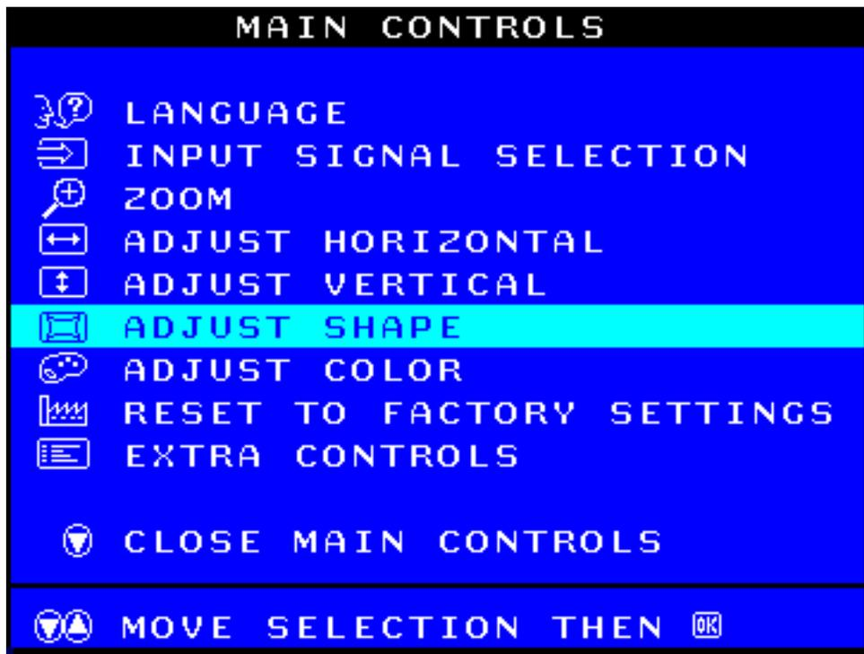
3) Press the
