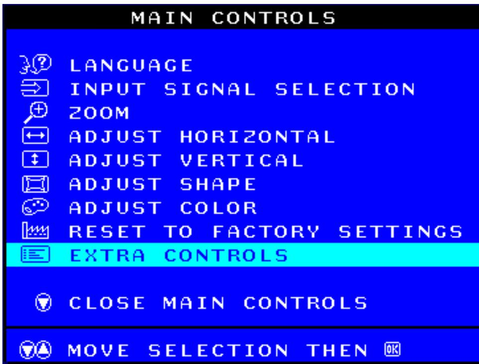
3) Press the
