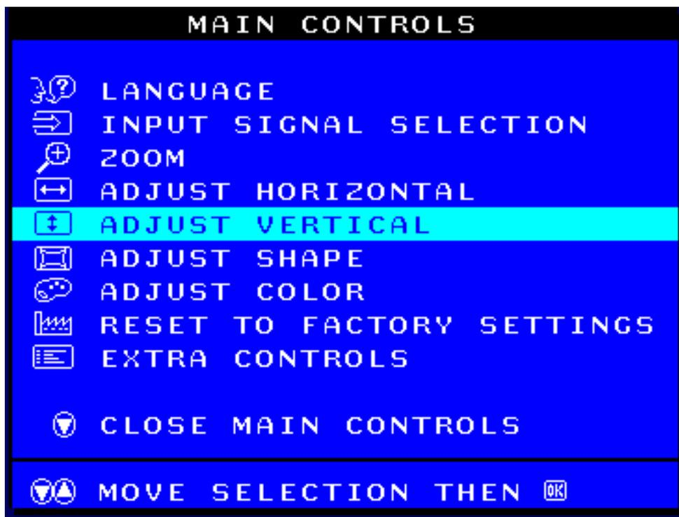
3) Press the
